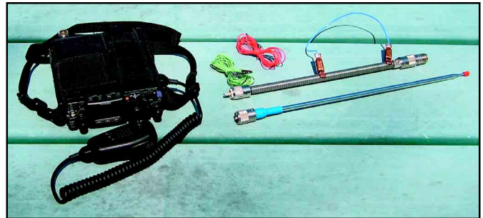
Figure 2—The completed FARApole antenna, dismantled, but ready for installation. The wire bundles are counterpoise radials that will be attached to the transceiver’s ground terminal. Note the right-angle UHF connector at the rear of the transceiver. This will ensure that the vertical antenna is, indeed, vertical.
